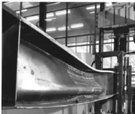
Figure 2. Vertical web buckling.
